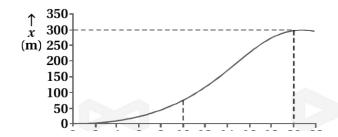
Picks up speed till t = 10 s and thereafter moves with uniform speed till t = 18 s. Then the brakes are applied and the car stops at t = 20 s and x = 296 m. The position–time graph for this case is as above.
