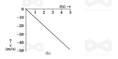
Velocity of object falling freely, v = -gt. Thus, graph (b) is obtained for  $v \to t$ .
